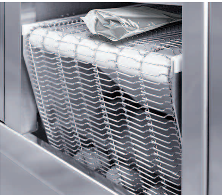
Fully automatic belt dryers (here with stand-up pouch) dry and cool separated products using targeted air routing.
