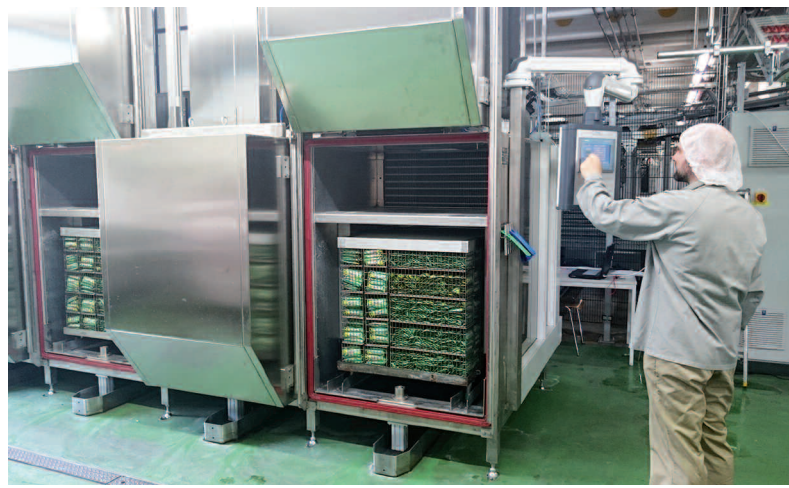
This classic batch dryer may also be used for pharmaceutical products.
