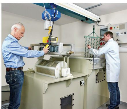
Drying Tests in Harter Pilot Plant Station for System Layout and Design
