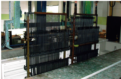
Rack entering the drying trough
