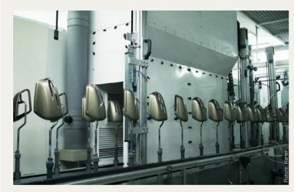
The low temperatures of the new paint drying system reduce the stresses on the plastic parts
