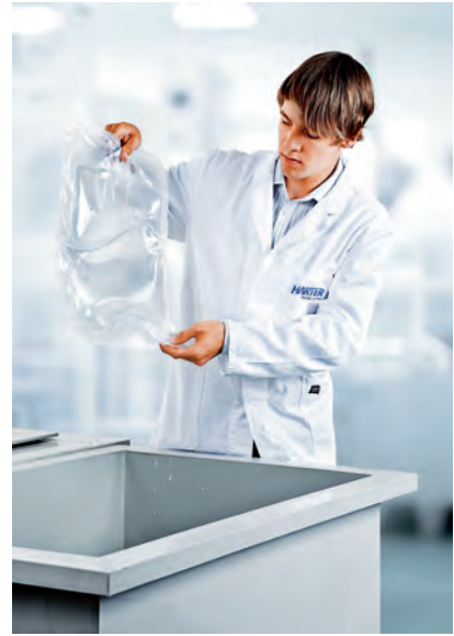
Fig. 7: Trial drying of infusion bottles in the Harter pilot plant station to determine parameters such as temperature, air speed and air paths.
