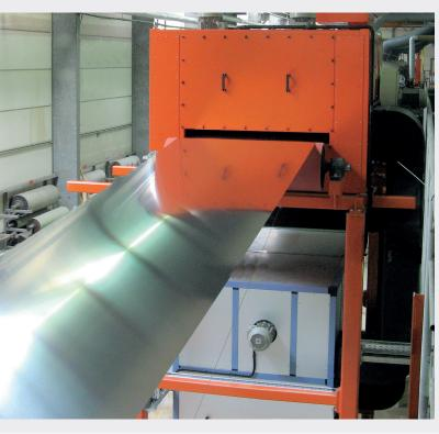
Rapid results – aluminium strip leaves the drying tunnel perfectly dry after two seconds.
