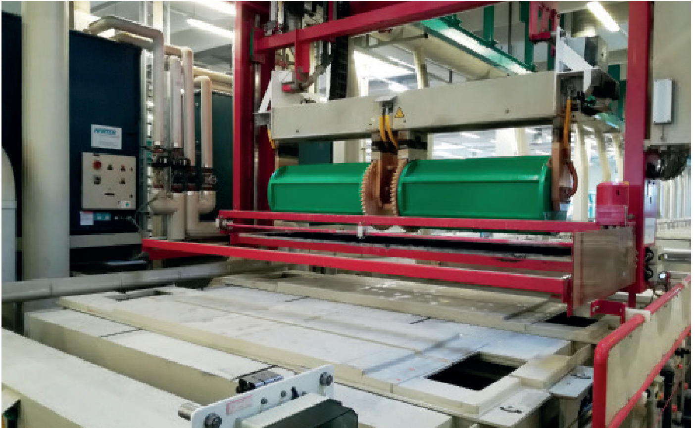
Fig. 1 – Complete, gentle and energy-saving drying of bulk material in a barrel dryer with minimal intermittent movement at a temperature of 70 °C
