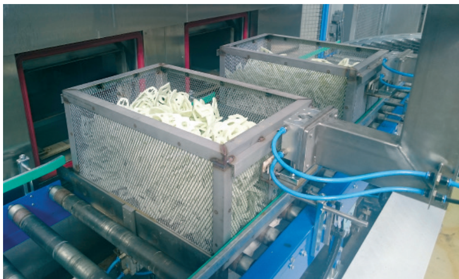
Fig. 3 – Combined drying-cooling continuous dryer
