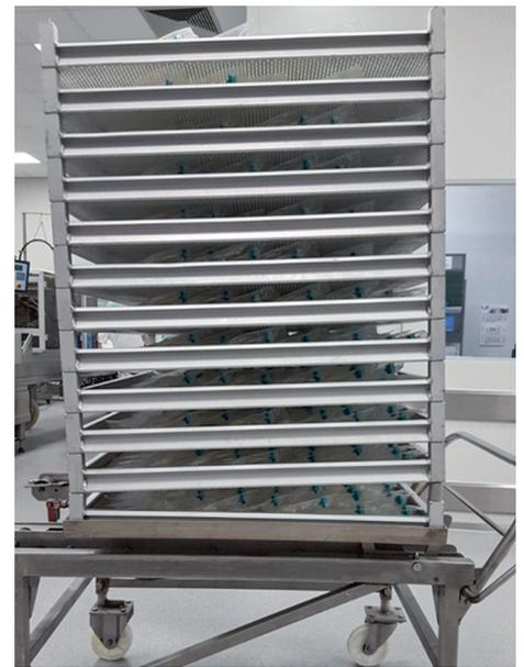
Series of tests showed that for successful drying the trays had to be inclined.
