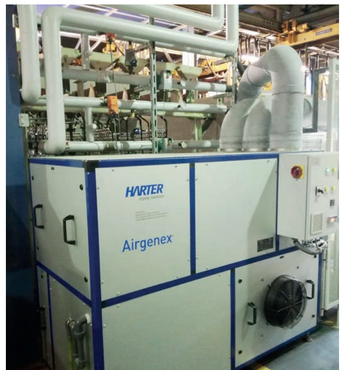
The Airgenex dehumidification module provides the required process air
