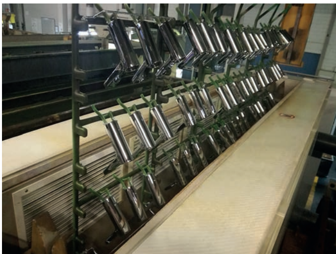
Fittings with complex geometries entering one of the three dryers
