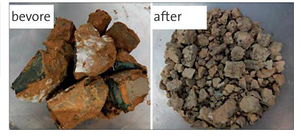
Tests are conducted in the HARTER pilot plant station to determine the drying response of the sludge and the drying parameters to be used.
