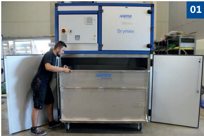
01 Drymex M4 dryer processes one ton of sludge a day
