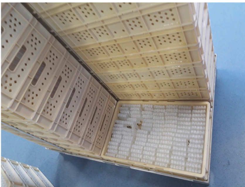
Fig. 1 – Following sterilization, ampoules in baskets stacked on pallets are rinsed completely, dried perfectly at 60 °C and then cooled to 30 °C ± 5 °C. (All illustrations by courtesy of Harter)
