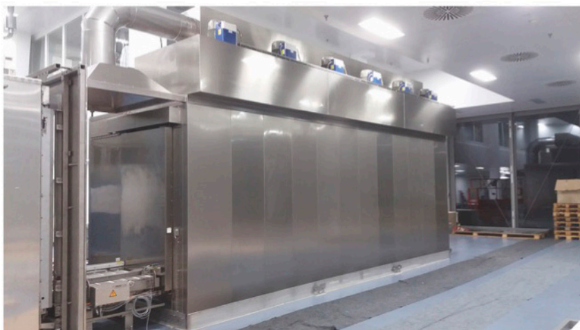
Fig. 2 – The fully automated system rinses, dries and cools. It is a closed air type with extremely low energy consumption and carbon emission.
