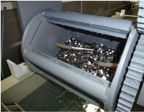
It takes no more than three minutes to dry the various carbide metal items loaded in four baskets.
