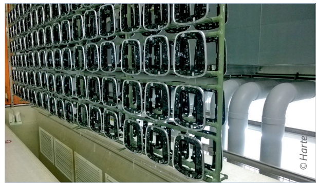
Fully Loaded Rack upon Insertion into Dryer
