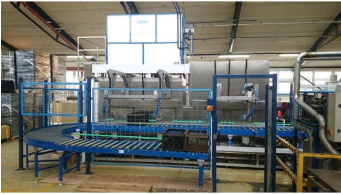
The compact dipping and drying machine. The dehumidification unit is located above the drying chamber to save space.
