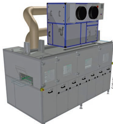
Baskets of bulk material pass seven combined air blowing/air recirculation drying stations inside the drying tunnel
