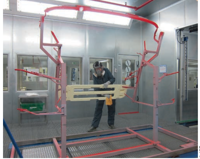
To minimize water input into the downstream paint coating process parts are finish shammed if required.
