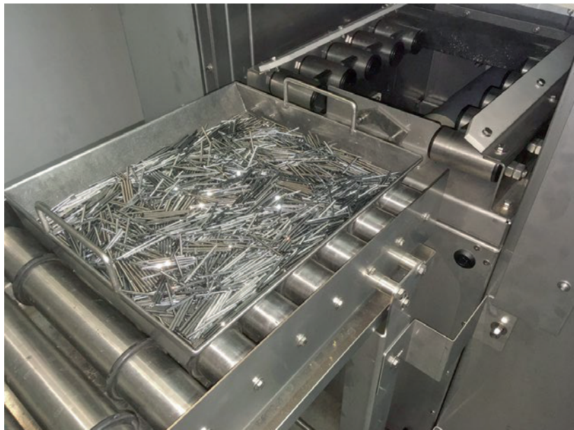
Baskets with hard metal rods entering the dryer. The rods are dried completely and stain-free within three minutes at 45 °C.
