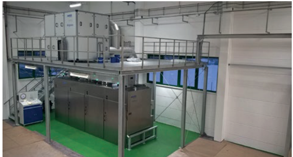
■ Fig. 2 – Almonds in containers are dried to a residual moisture content of less than 5 percent for subsequent grinding.
