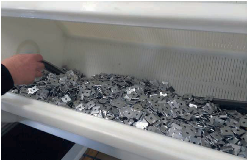
Fig. 2 – Comfortable in-line drying is state-of-the-art. The bulk material shown is dried in a reliable and gentle way at a temperature of 75 °C for eight minutes.
