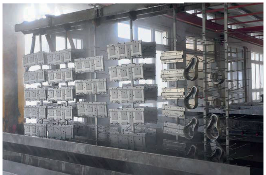
Fig. 1 – Racks entering the dryer after anodizing. Components are dried completely and stain-free at a temperature of 65 °C for 15 minutes.
