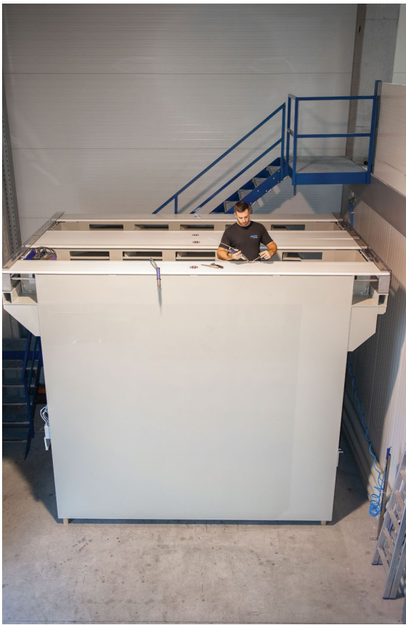
Large size rack dryers can process aluminium components as wide as 6 m to become completely dry (photograph showing an example for drying 4.4 m max. widths)
