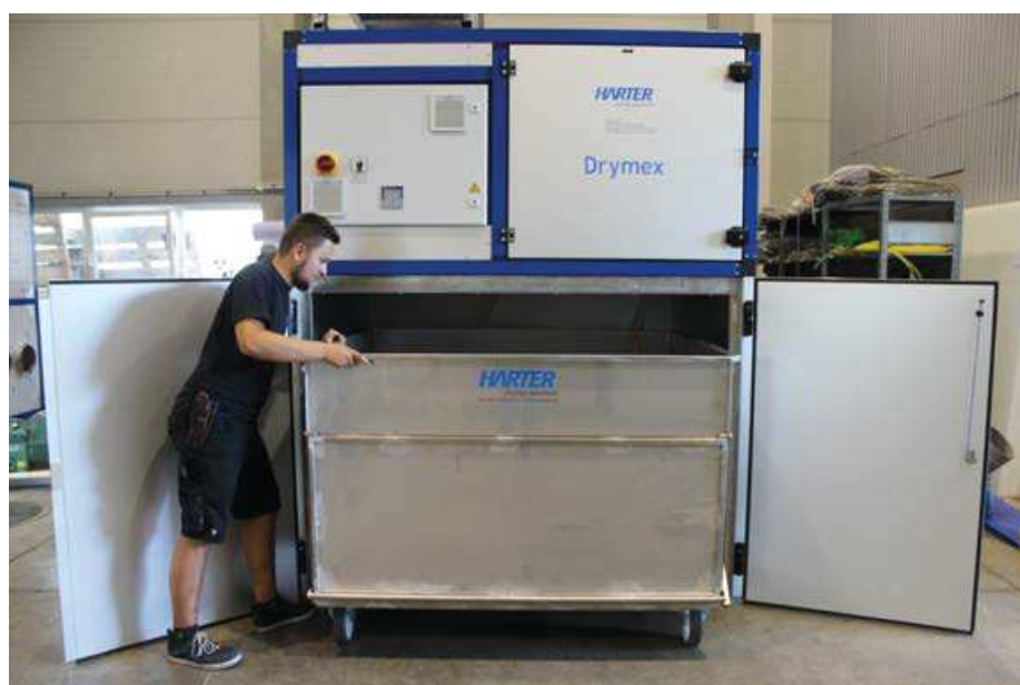
Fig. 5 - Standard sludge dryer for drying 1,000 kg of sludge a day
