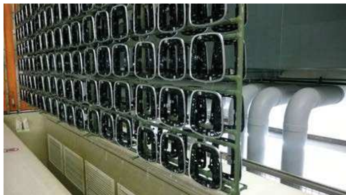
Fig. 1 and 2 – Racked metal and plastic items are gently processed in rack dryers to become completely dry within the specified cycle times.
