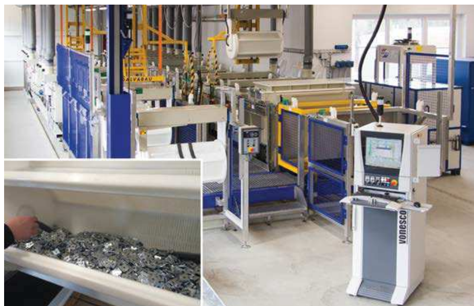
Fig. 3 - Convenient and reliable in-container drying of bulk material. In-barrel drying is state-of-the-art today.
