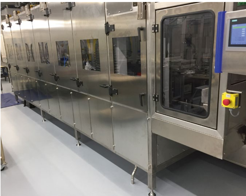
Items in bulk or separate electrical components are fully dried at 60 °C under cleanroom conditions.
