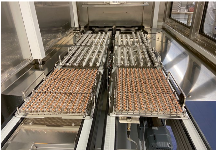
There is a signal by a traffic light. All eight baskets can be moved forward, one after another, at the push of a button so that the worker may carry them off with ease.
