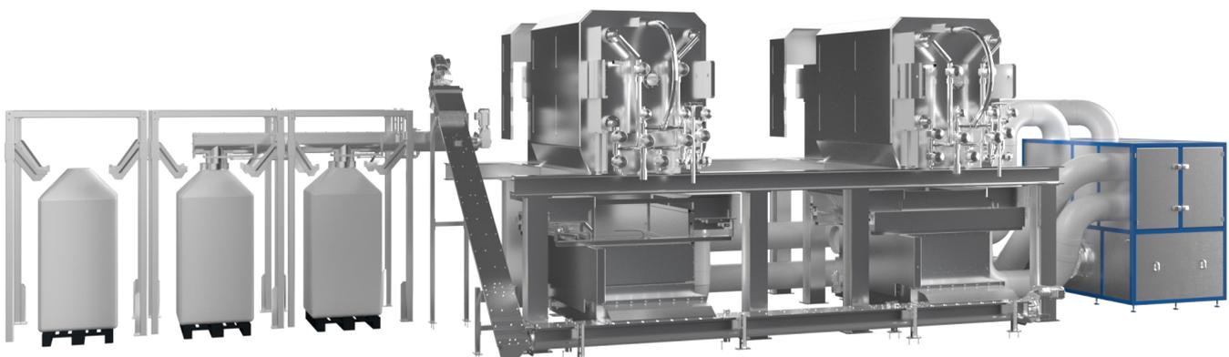
*The two chamber filter presses release sludge to fall into the drying containers underneath. A conveying system automatically transports the dried sludge from the containers to the big bag filling station. The dehumidification module to condition the required process air is shown on the right.*
