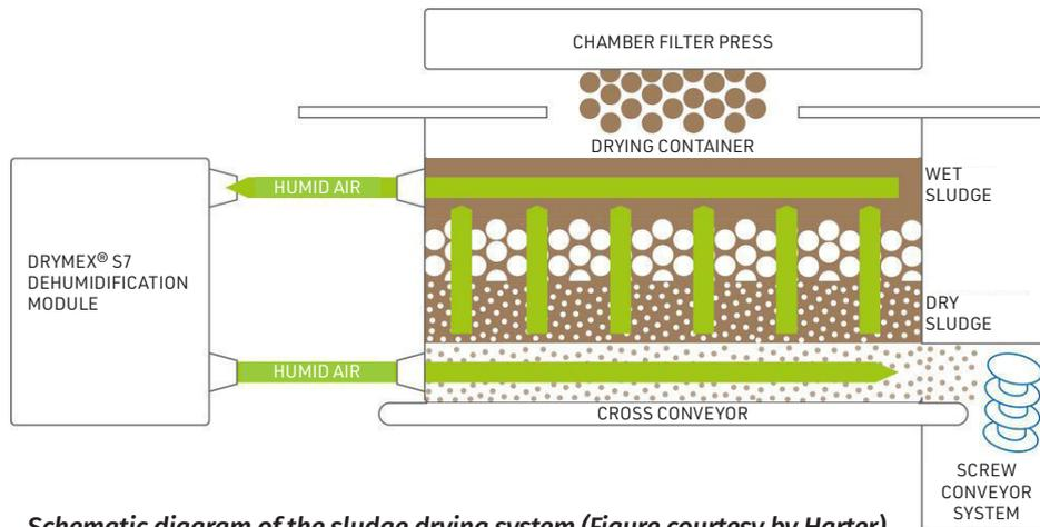
*Schematic diagram of the sludge drying system (Figure courtesy by Harter)*
