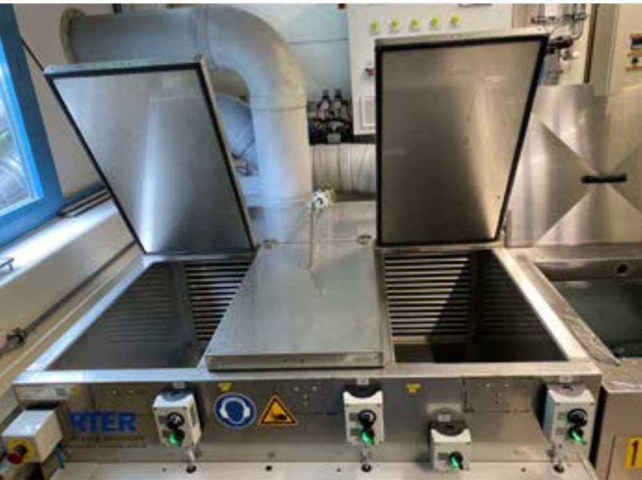
Jabil's new basket dryer features three chambers for two baskets each. Its highlight is special air routing. (Photograph courtesy by Harter)
