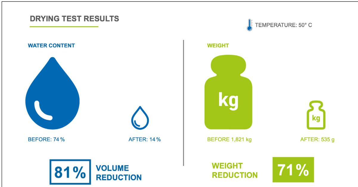
Fig. 1 – Drying test results demonstrate the sludge volume and weight reduction potential. This forms the basis for calculating the pay-off period.
