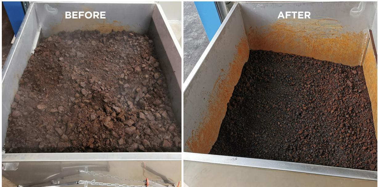
Fig. 2 – Drying substantially reduces sludge volume, weight and, above all, disposal cost.
