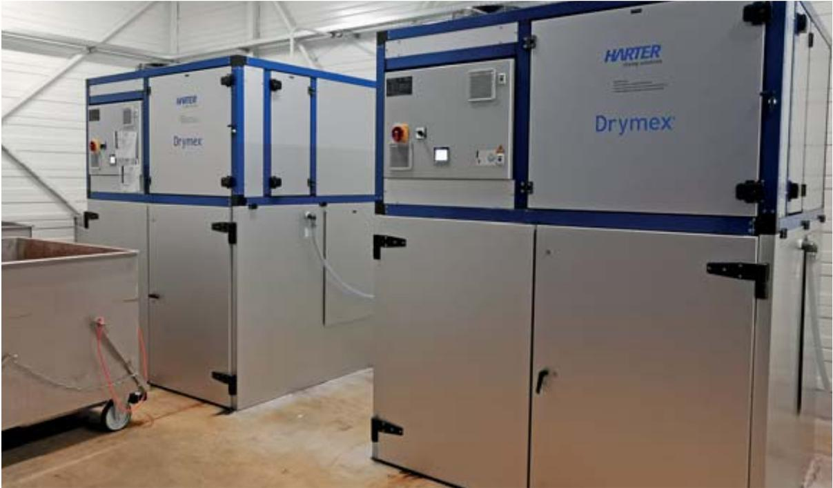
Fig. 3 – Type M5 dryer with two containers each. Each container has a useful volume of 1.5 m<sup>3</sup>.
