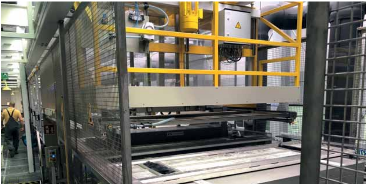
Each drying station features an automatic lid system to retain the precious heat. Drying takes place in a closed air system.
