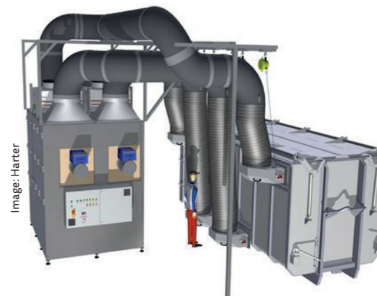
Drying in the roll-off container directly under the chamber filter press
