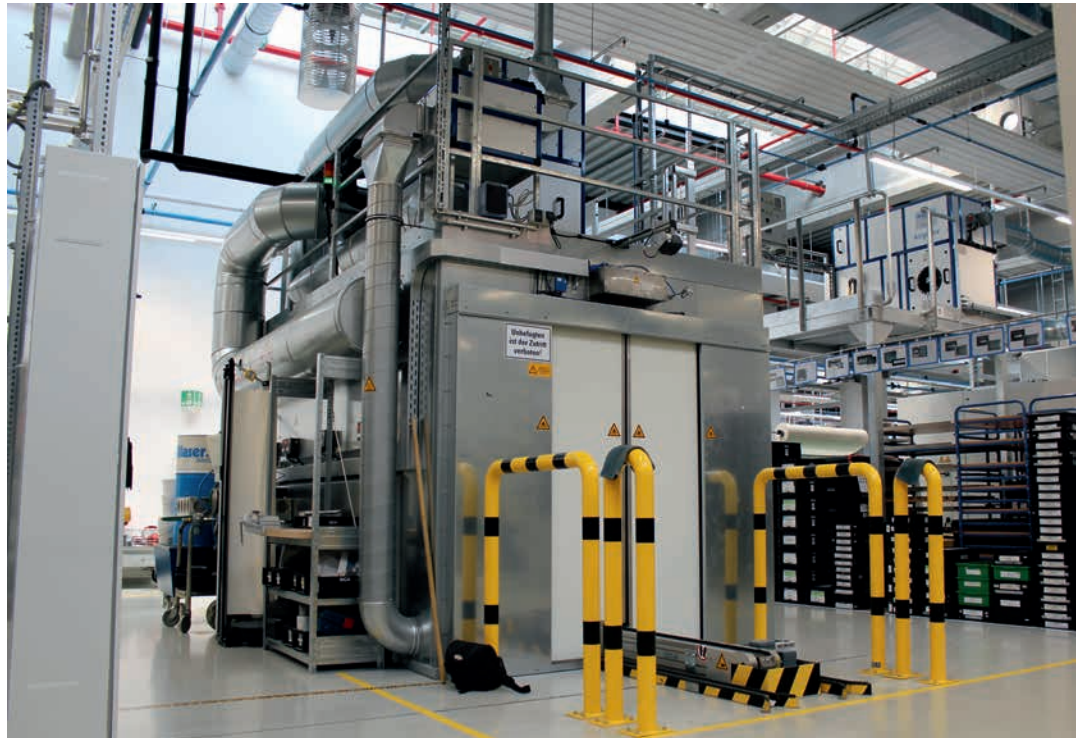
The "Airgenex" combined system is used for air drying and curing
