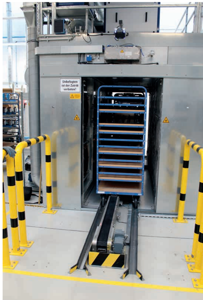
The trolleys are conveyed into the drying chamber
