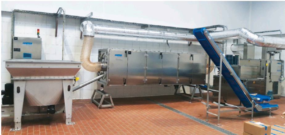
The system customized for Maintal Konfitueren is a continuous barrel dryer with a cooling tunnel, conveying system, dispensing hopper and dust separator. The final product is a premium organic wild rose oil.
