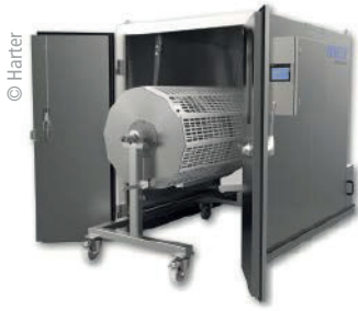
Fig. 2: Horseradish lateral shoots are upgraded by drying and then sold to the pharmaceutical industry.
