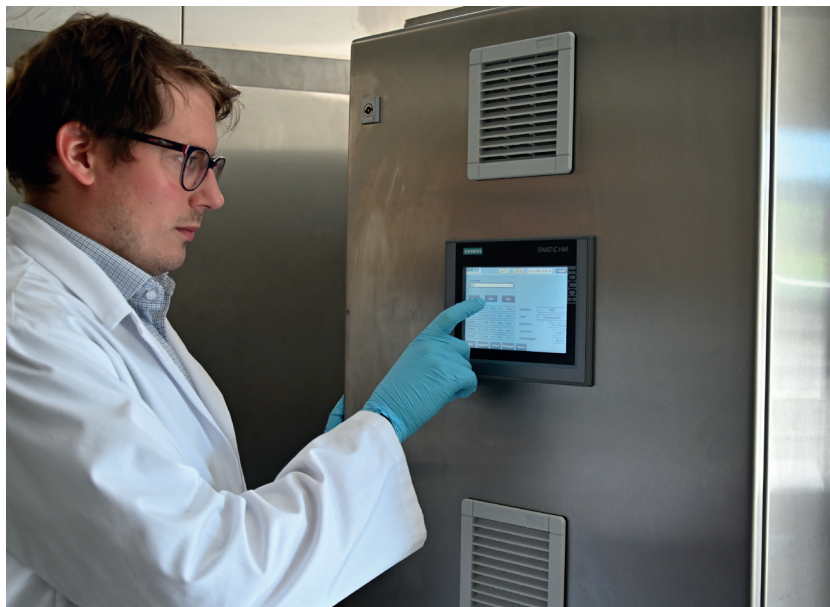
For delicate products, five phases with different parameters may be specified in the individual drying profile stored in the controller. (Images: Harter)
