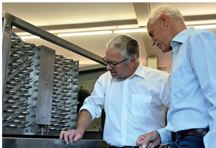
The highly efficient heat exchanger system integrated in each dryer heats and cools the process air at two stages.
