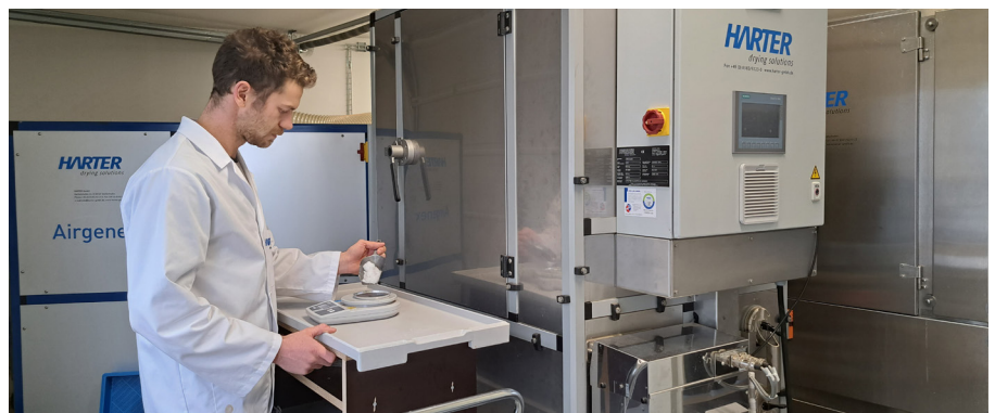
Products are tested for feasibility and drying properties in Harter's Test Center – in this case coarse-grained table salt. Various dryers are available for testing.
