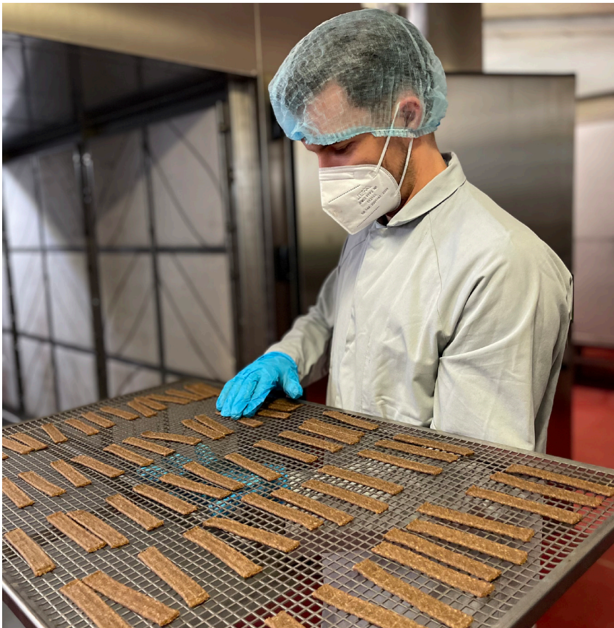
Managing Director Philipp Hibler inspects dried material for conformity with defined quality features including the defined residual humidity, the desired consistency, and a uniformly dry product.
