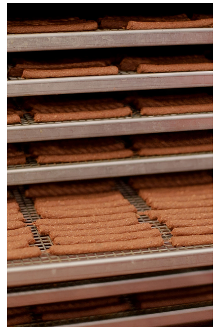
Residual humidities below 10 percent were obtained in tests at 50 °C to 55 °C. This corresponded to the desired consistency. Defined temperature limits enable exact dry matter contents to be achieved. Absolute process reliability is thus ensured.
