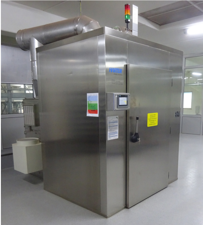
The stainless steel chamber dryer processes the tea ingredients to obtain the desired four percent residual humidity within six hours. Right: Condensation drying meets highest demands; pomegranate peel is being processed here.
