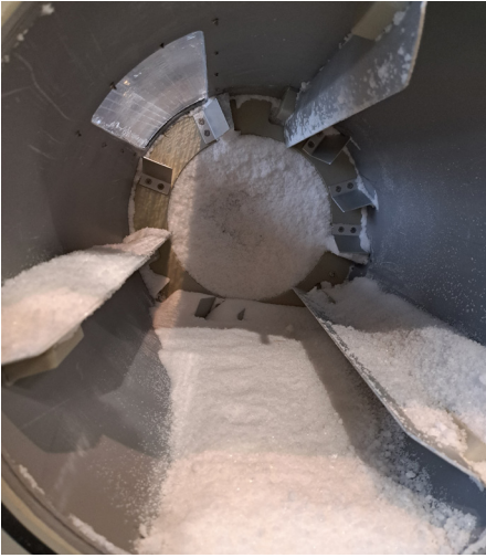
■ Fig. 2: Table salt was dried in a barrel slightly rotated continuously to obtain a uniform less than two percent residual humidity. The time required for the process was only 40 minutes.
