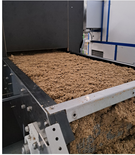
■ Fig. 3 – This example shows brewer's spent grain on a conveyor belt. All such tests are used to determine parameters such as bulk height, belt and air speed. They provide information about where to place drops, how many drops to use and, ultimately, the ideal design of the entire drying solution.
