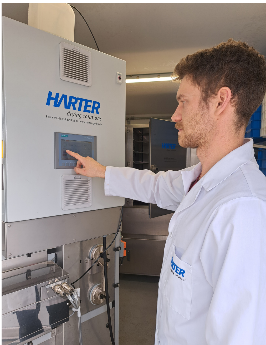
■ Fig. 1 – The control board of the chamber dryer in the Test Center gives Fabian Bauraquick and easy access for varying the parameters for the individual tests runs. The best parameters obtained are ultimately stored as a recipe.
