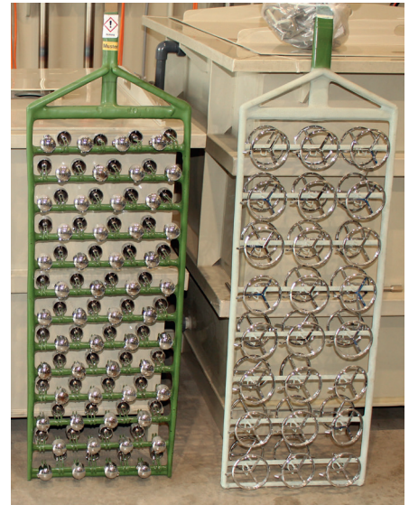
Racks holding items to be dried in preliminary condensation drying tests
