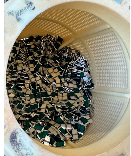
To dry minute parts in finely perforated baskets successfully, targeted routing of the unsaturated process air is key. Testing in the in-house Test Center is the pathway to arrive at a viable drying solution for bulk items of various sizes and quantities.
