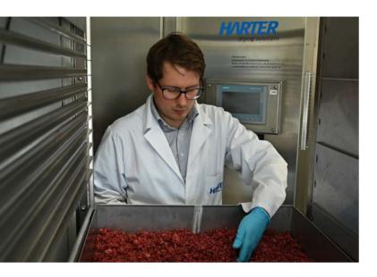
Our services include series of tests in our pilot plant station. This appears to be the best method for determining the parameters for successful drying. We run these tests – which you are welcome to witness – to identify the best temperature, humidity, drying time, air speed and airflow.
