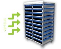
Products which can be dried in bulk may be loaded 175 mm max. high. The direction of airflow is modified such that the air entering the chamber horizontally is diverted to flow vertically through the pans to finally leave the chamber horizontally again. This is the only way to ensure uniform drying of bulk products.
