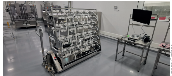
Two carts for mounting the oxygenators are associated with each dryer. These carts are special builds to accommodate the complex and different geometries.
