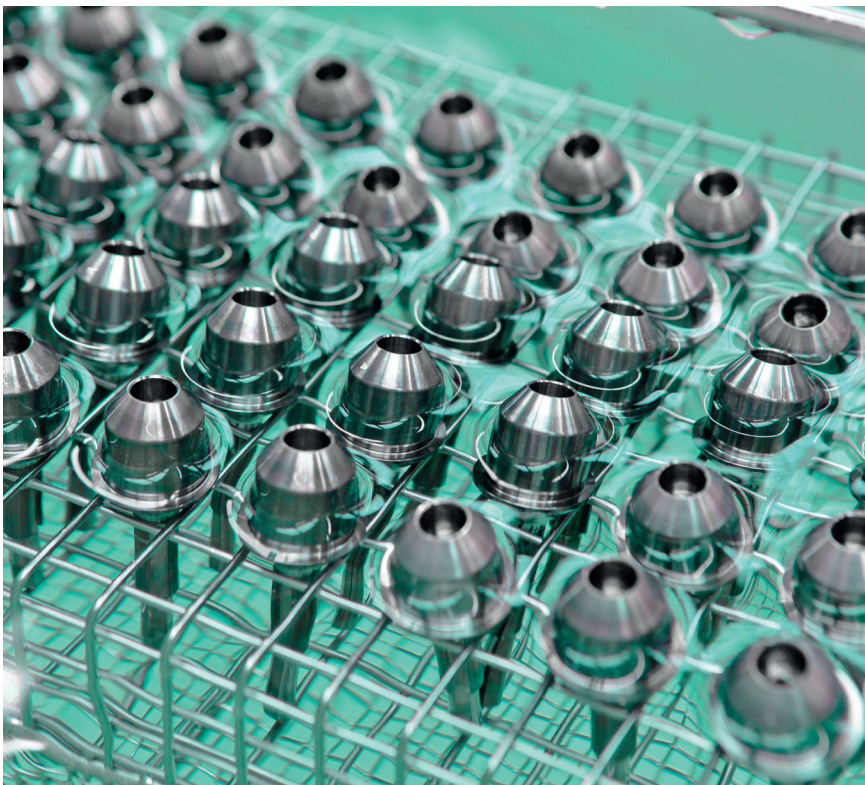
Appropriate cleaning and complete drying are requisite for passivating metallic components for implants and instruments.
