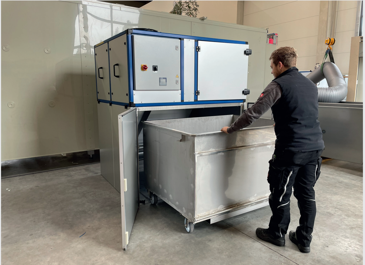
Fig. 2 - Filter pressed sludge is dried to a residual humidity of about 15 percent. The integrated heat pump lowers the power demand for the drying process, thus adding to the cost savings.
