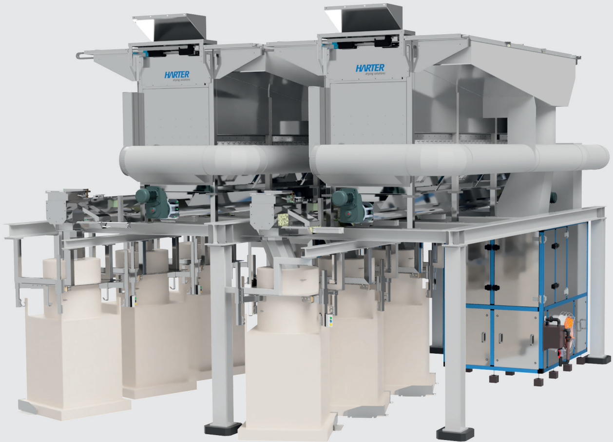
Fig. 3 - The fully automatic facility consists of two drying containers, two heat pump modules, and a screw and belt conveyor to the big bags. Following drying at 50 °C for about 20 hours, the dried sludge is placed in the furnace for recycling.
