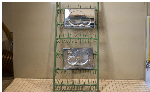
Drying tests revealed the requirement for additional air blowing of the water entrapping plastic plates.
