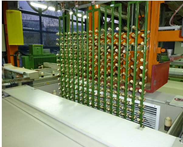
Components of door locking systems are reliably processed to become dry and stain-free within 10 min at 70 °C.
