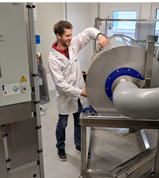
Fig. 2 – Baur uses the barrel returned from off-site testing for test drying coffee pomace. The very fine particles require continuous mixing for uniform drying.
