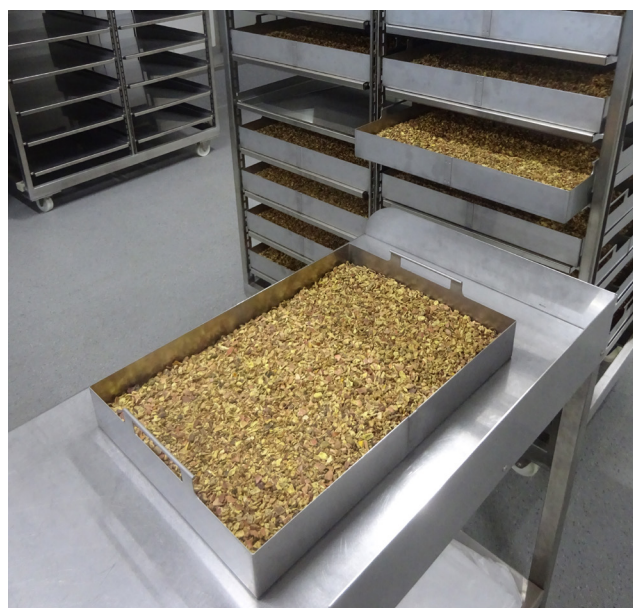
Fig. 1 Drying of herbs and fruit parts to become precious and aromatic infusion ingredients is accomplished with a versatile chamber dryer. Absolutely uniform drying takes place at 50 °C in a closed air system - without producing any exhaust air.
