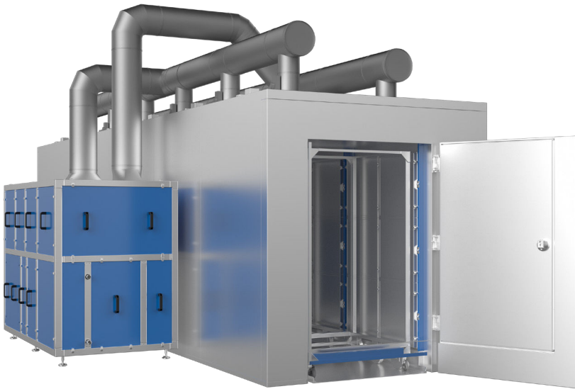
The 8-chamber dryer is designed to process daily batches of about 1,500 kg of sausage meat placed on Inter carne's existing trolleys
