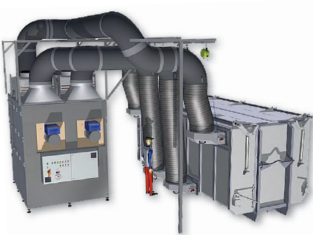
Container dryer – particularly suitable for chamber filter pressed sludge
